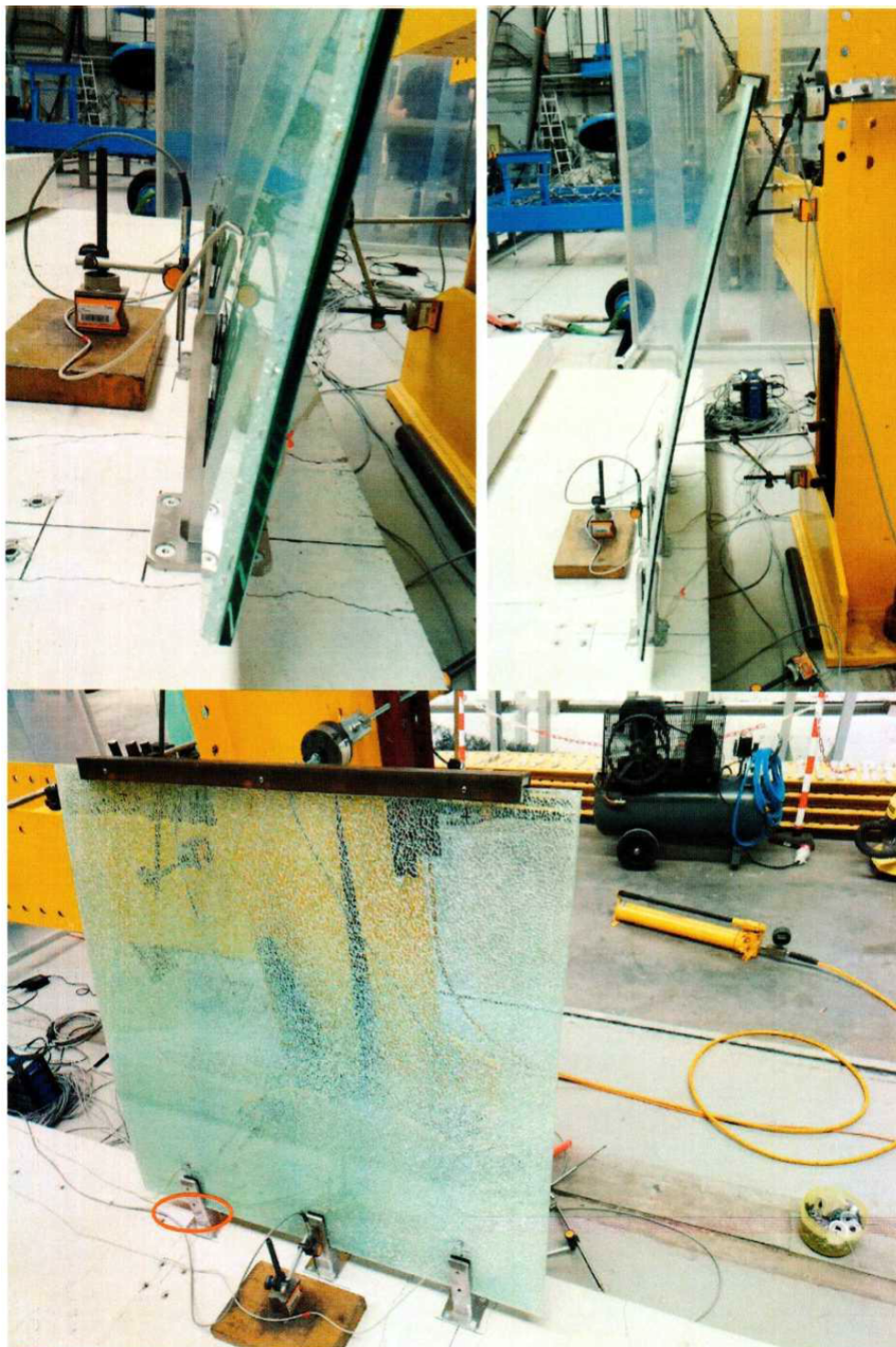
Deformed railing under a load of glass collapse 3x SPIGOT
