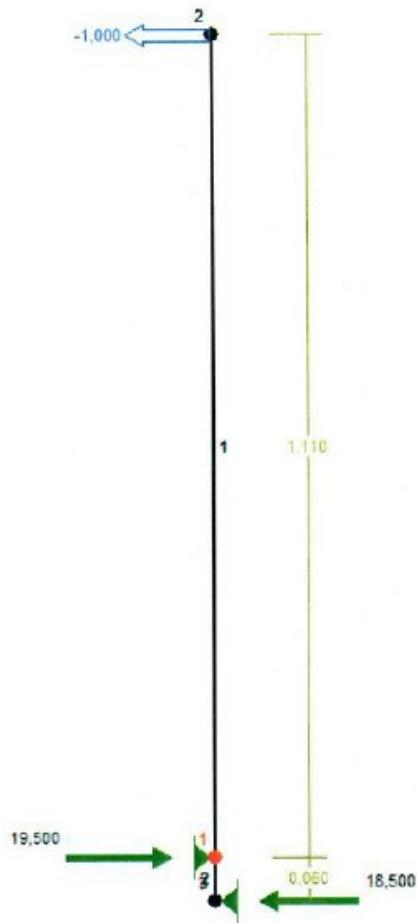
Specification of powers acting on the inserts transferring the load on the profile walls
