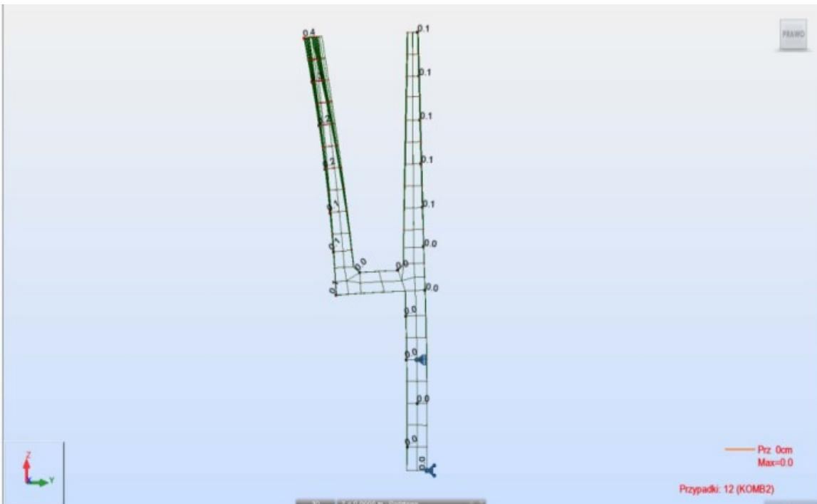
Maximal deflection of the vertical profile wall equals **4mm**.
