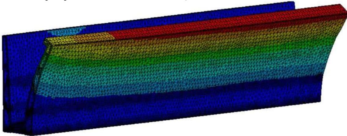
The maximum deformation of the profile is 1.26 mm.
