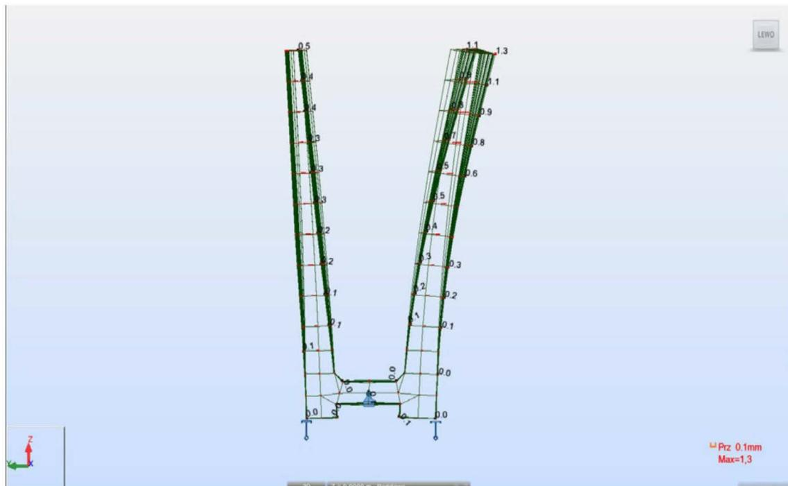
Maximal deflection of the vertical profile wall equals **1,3mm**.
