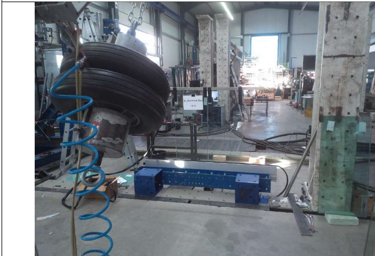
Test setup 4 Impact test with drop height \Delta h = 700 mm on P1 → no damage
