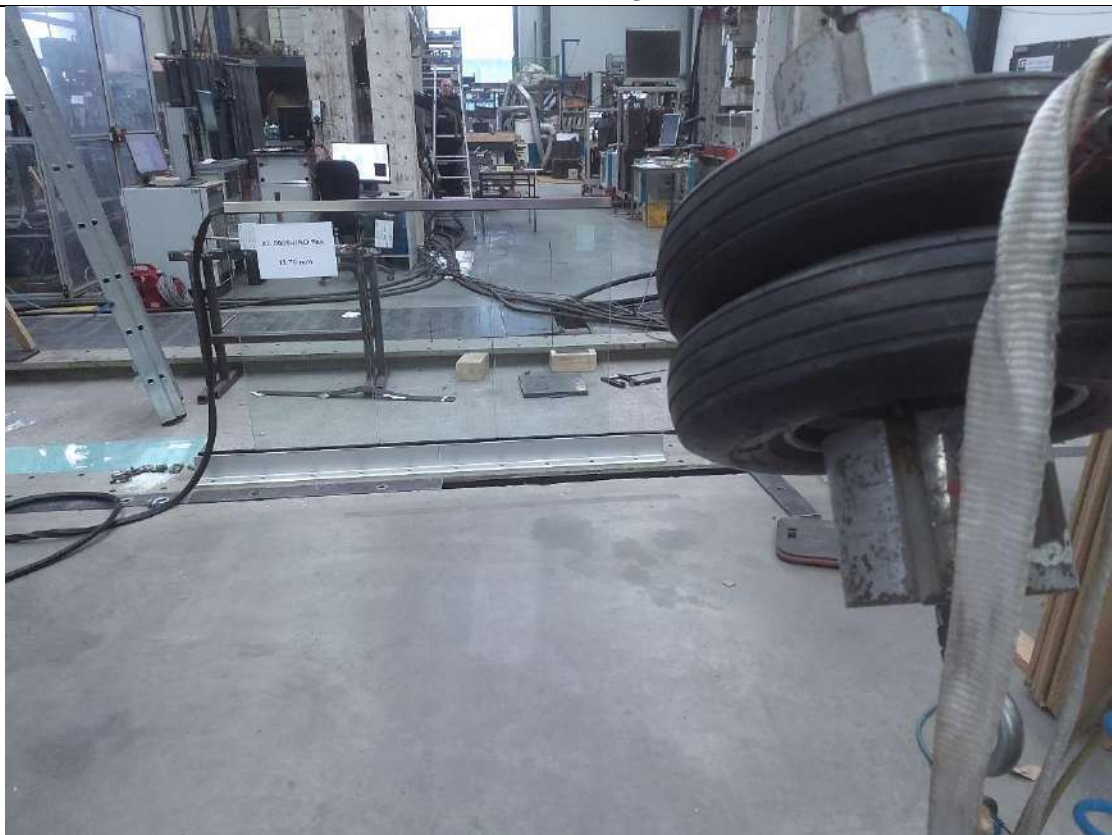
Test setup 2 Impact test with drop height \Delta h = 700 mm on P2 → no damage
