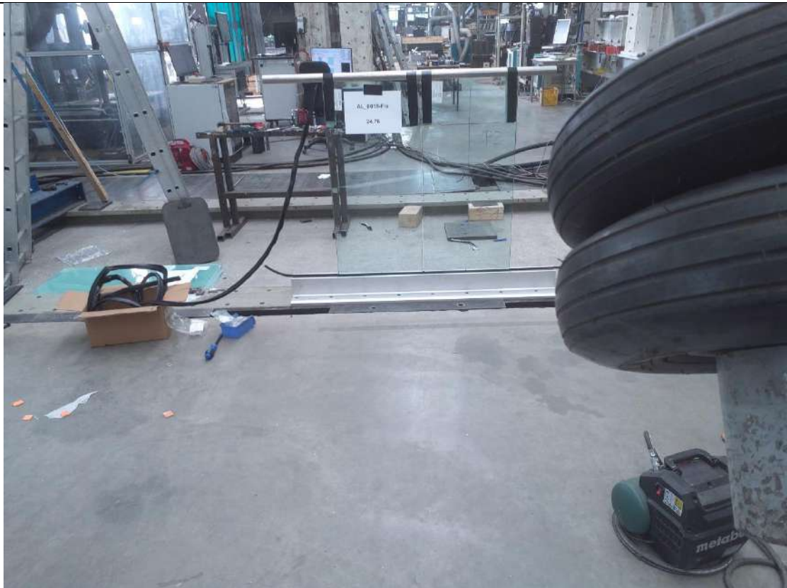
Test setup 5 Impact test with drop height \Delta h = 700 mm on P2 → no damage
