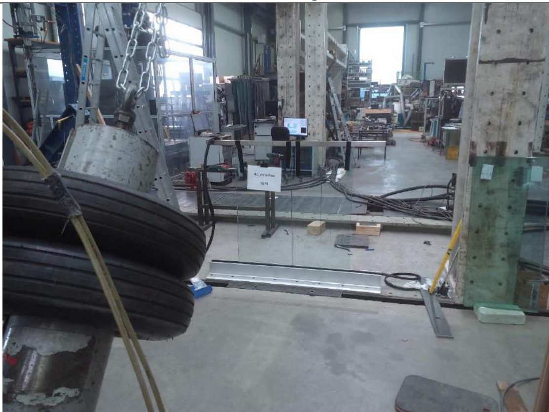
Test setup 6 Impact test with drop height \Delta h = 700 mm on P1 → no damage
